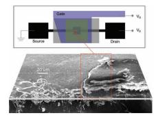
A hybrid sheet-based manufacturing approach for organic electrochemical transistors is reported. It combines screen and inkjet printing with a self-aligning laser ablation step.
