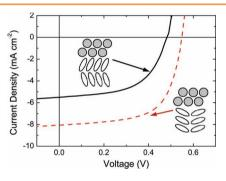
The effect of molecular orientation on the photovoltaic processes of a polycrystal-line zinc phthalocyanine/C<sub>60</sub> heterojunction are explored. Not only is absorption affected by molecular orientation, but exciton transport and charge transfer efficiency are also influenced and these processes account for an increase by nearly a factor of two in the efficiency of the bilayer cells studied.
