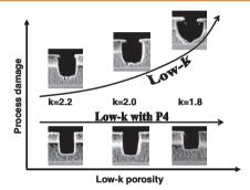
Protecting the porosity of ultralow dielectric constant (k) materials allows for limitation of the processing damage to a constant minimal level, independent of the porosity. This trend holds true on both blanket wafers and patterned structures, highlighting how the post porosity plasma protection (P4) can allow the extendibility of actual semiconductor manufacturing processes to future highly porous dielectrics.
