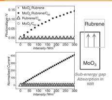
A simple approach to achieve near-infrared electric power generation using the interactive charge-transfer complex formed between molybdenum (VI) oxide (MoO<sub>3</sub>) and the wide-energy-gap 5,6,11,12-tetraphenylnaphthacene (rubrene) is presented. An intermediate state induced within the energy gap of rubrene leads to sub-energy-gap absorption and photopower generation.
