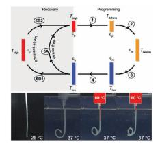
Biomedical applications often require intelligent devices that can perform self-sufficient shape changes or can be fixed in an adapted geometry. The working principle of temperature-memory catheters based on copolyesterurethanes containing poly(\omega-pentadecalactone) and poly(\omega-caprolactone) segments as controlling units for the temperature-memory effect are explored. The response temperatures of such polymers can be adjusted in a range relevant for biomedical applications.
